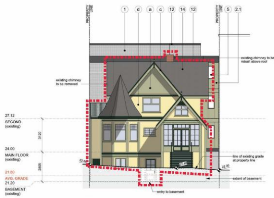
3 FORT STREET (FRONT) NORTH ELEVATION Scale: 1:100
