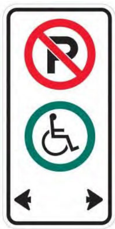
Figure 2: Motor Vehicle Act Regulations Division 23 Schedule 2 Sign. The sign must be at least 60cm x 30.
