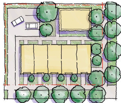
Example showing accomodation of a corner townhouse with rear-yard parking while still accomodating yard space for individual units along with required open site space and tree planting space
