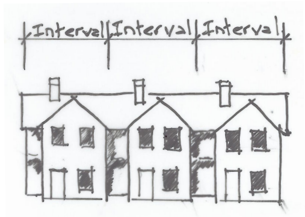
Consider articulating facades into a series of intervals to emphasize individual units and entryways, help break up the mass of larger buildings, and create visual interest along the street
