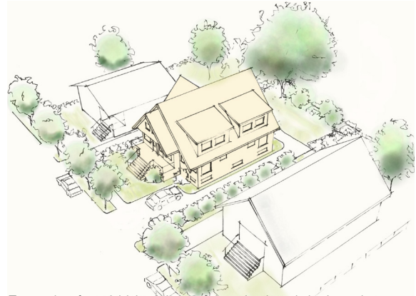
Example of a mid-block houseplex sited and designed to maintain the pattern of green front and back yards and oriented positively to the street.
