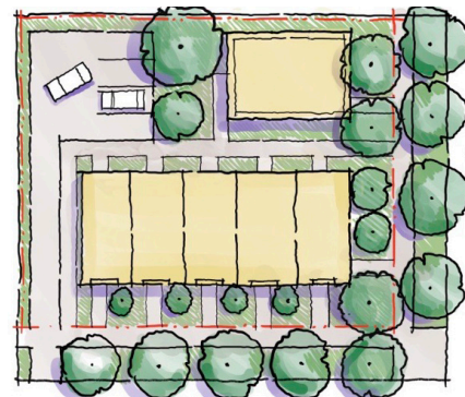
Example showing accommodation of a corner townhouse with rear-yard parking while still accommodating yard space for individual units along with required open site space and tree planting space
