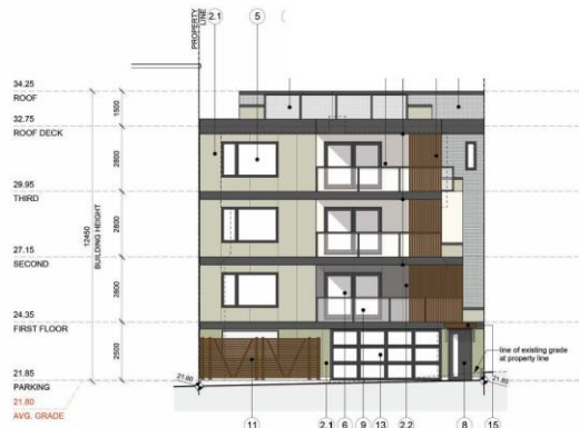
1 MEARE'S STREET (REAR) SOUTH ELEVATION Scale: 1:100
