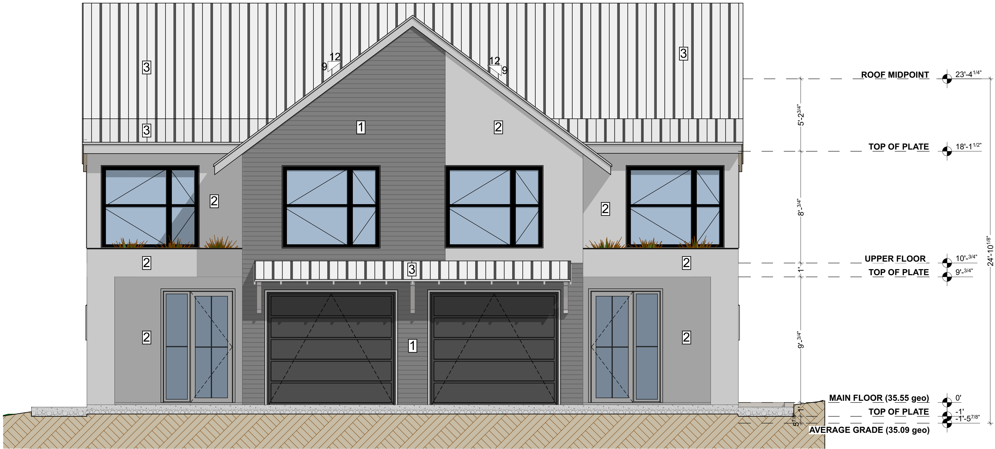
1 FRONT ELEVATION SCALE: 1/4" = 1'-0"
