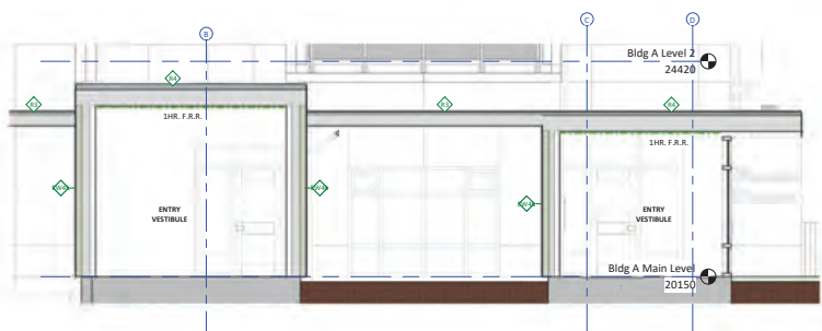
4 Building A Entry Vestibule Roof Section 1:50
