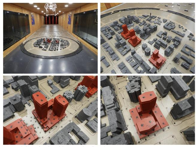
Image 2: Wind Tunnel Study Model - Proposed Configuration
