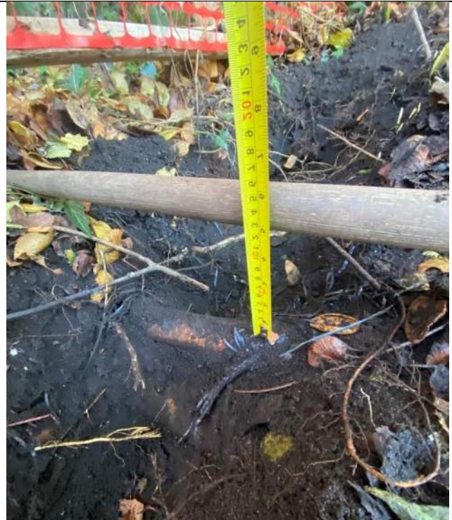
Photograph 2: 7cm root encountered at 2.8m from Southeast property corner (top of root approximately 13cm below existing grade).
