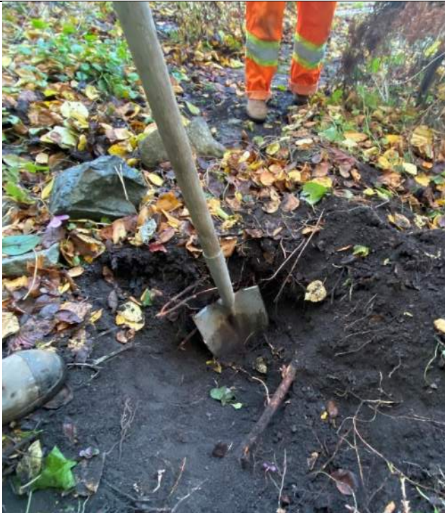
Photograph 1: 4cm root encountered at 4m from Southeast property corner (top of root approximately 25cm below existing grade)
