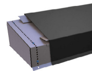
⑨ PRE-FINISHED METAL FLASHING - GREY
