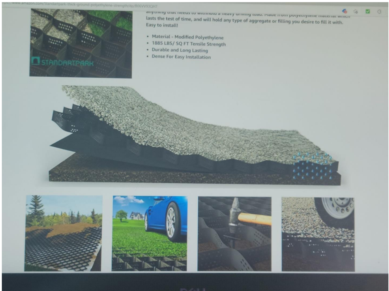
Figure #9 – Geogrid Path Design
