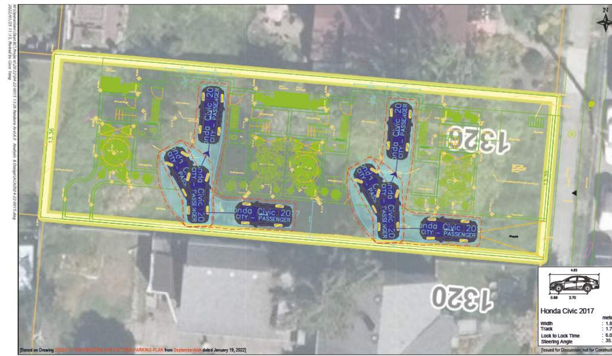
Exhibit 2 Unit 1 & 3 Parking Stall Accessibility - Inbound 1326 Pandora Ave Prepared by CY Scale 1:125 on Ledger January, 2022
