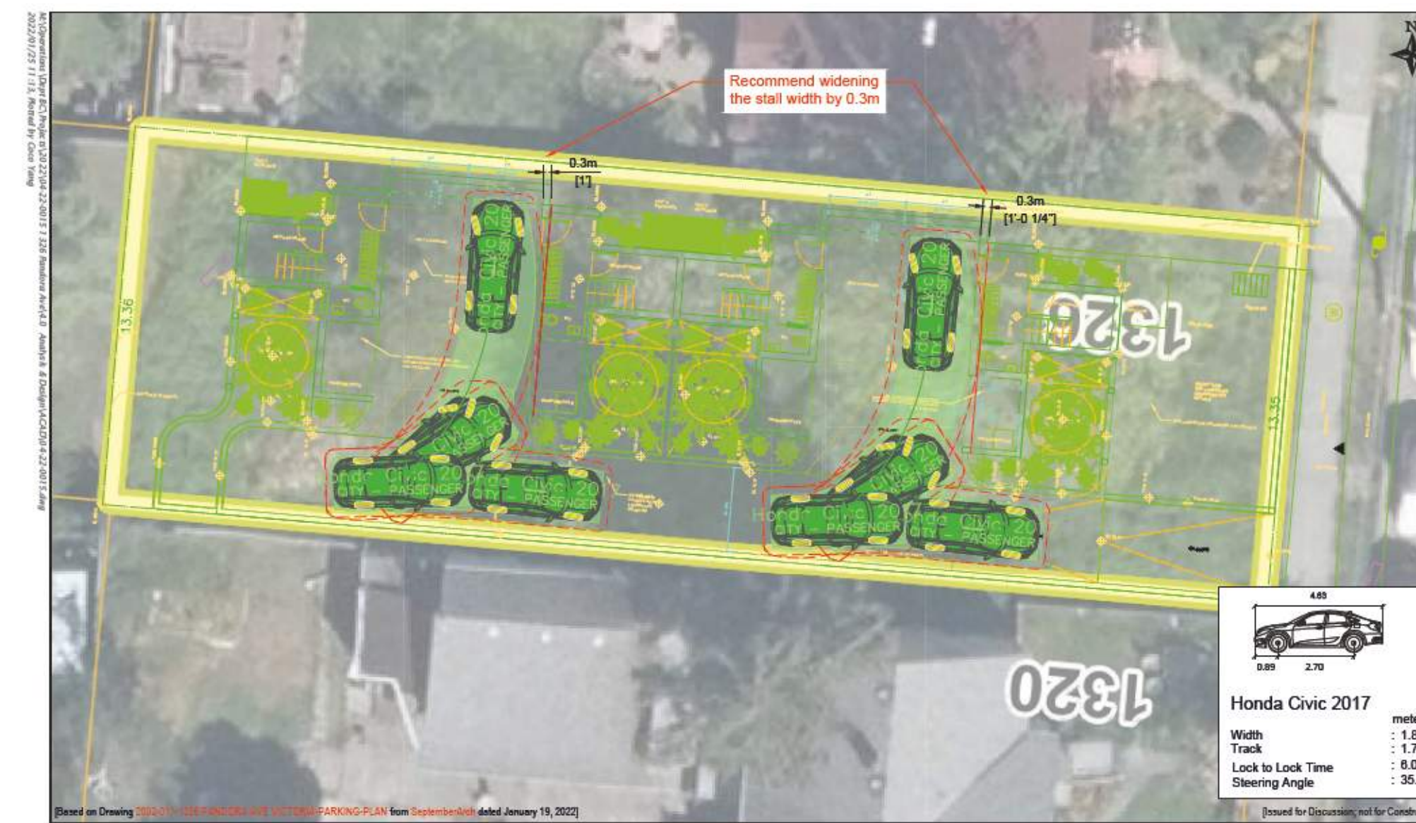
Exhibit 4 Unit 1 & 3 Parking Stall Accessibility - Outbound 1326 Pandora Ave Prepared by CY Scale 1:125 on Ledger January, 2022
