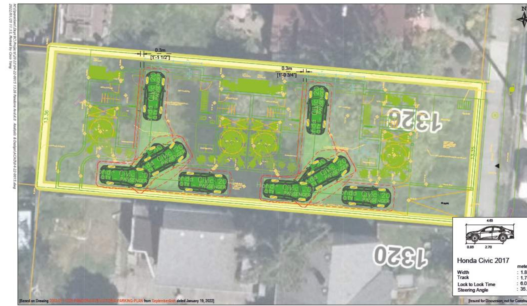
Exhibit 5 Unit 2 & 4 Parking Stall Accessibility - Outbound 1326 Pandora Ave Prepared by CY Scale 1:125 on Ledger January, 2022
