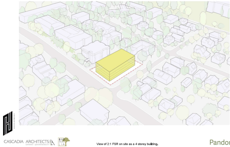
View of 2:1 FSR on site as a 4 storey building.
