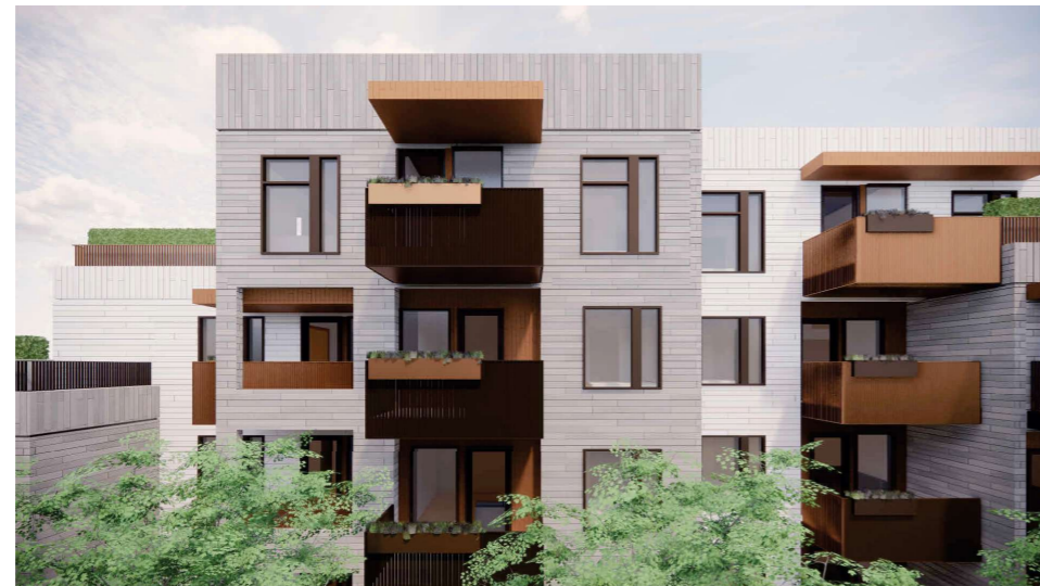
View from neighbouring top floor balcony showing privacy provided by angled guardrail pickets
