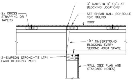
3 S1.3 1" = 1'-0" TYPICAL WALL TO TJI ROOF JOIST CONNECTION WHERE JOISTS RUN PERPENDICULAR TO WALL
