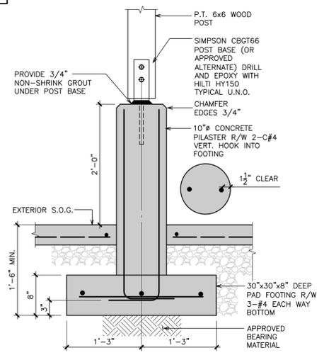
2 S1.3 1" = 1'-0" TYPICAL CONCRETE PILASTER DETAIL
