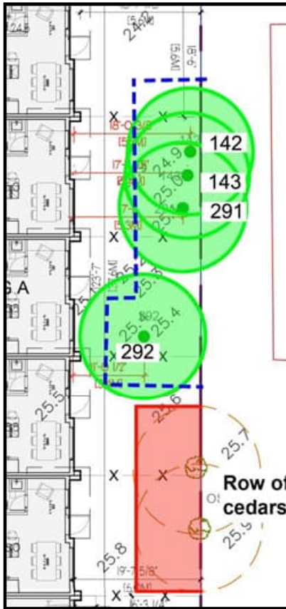
Figure 4. Fencing around trees 142, 143, 291, 292.
