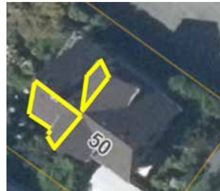
Possible areas for rooftop solar arrays
