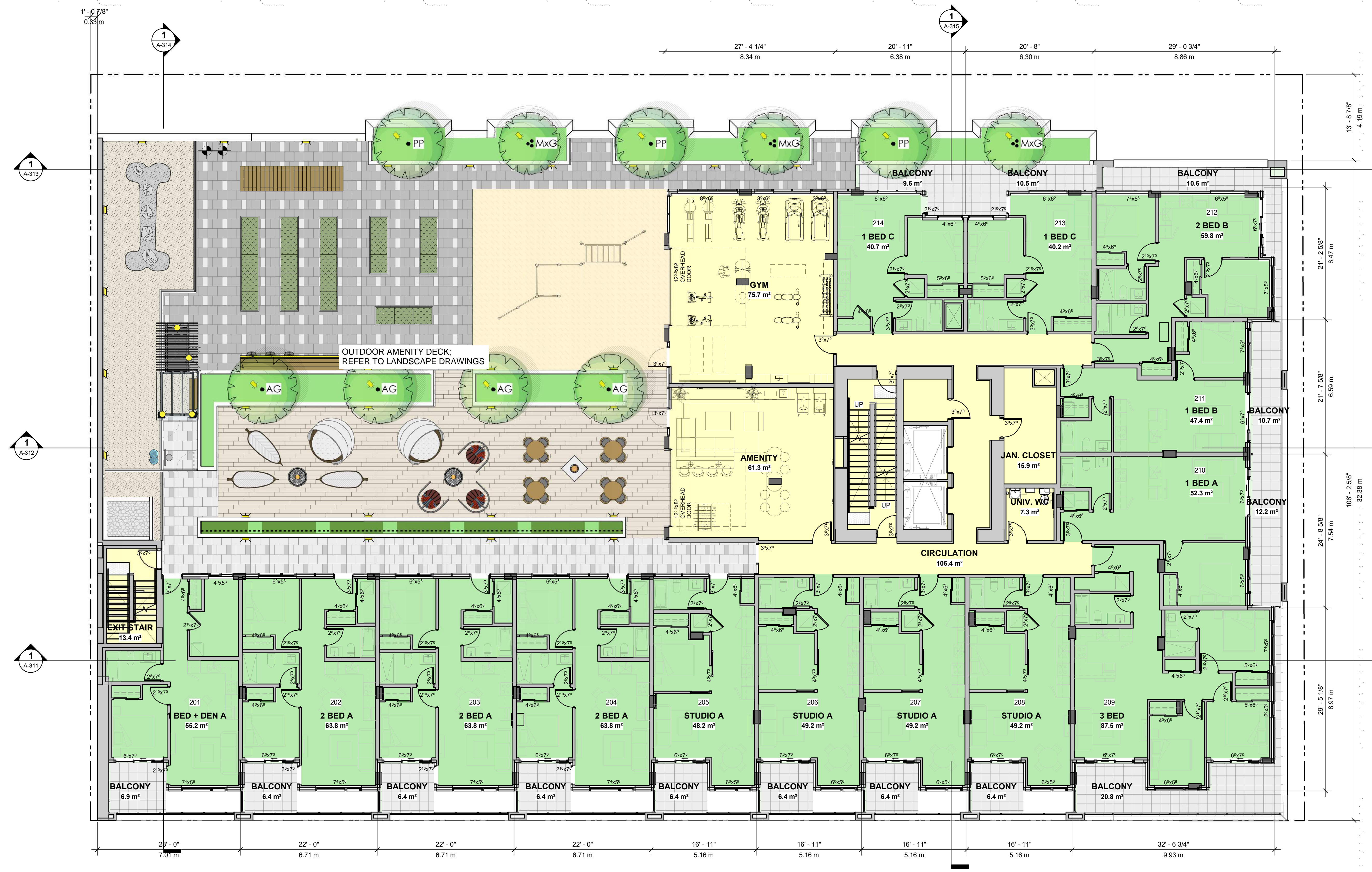
LEVEL 2 FLOOR PLAN SCALE: 1/8" = 1'-0"
