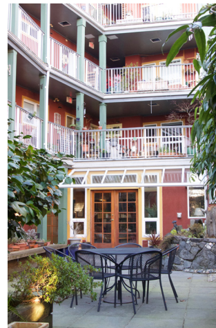
Single-loaded corridor form allows for improved livability at inside corners of an L-shaped residential floor in North Vancouver [Courtyard Architects - Quayside Village Cohousing; Image credit: xxx]
