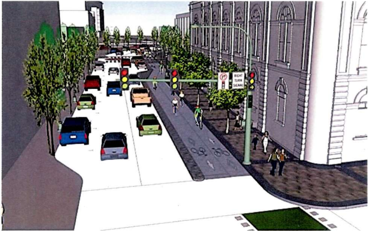
Figure 1 – Two-way protected bike lane (with signal changes) – Pandora/Douglas looking towards the Johnson Street Bridge
