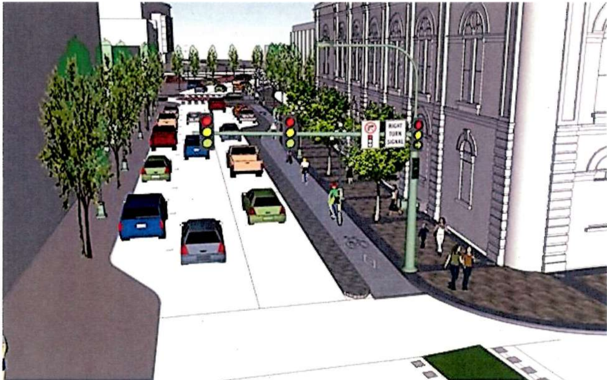
Figure 2 – One-way protected bike lane (with signal changes) – Pandora/Douglas looking towards the Johnson Street Bridge
