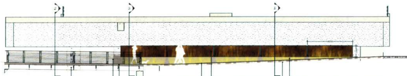
Figure 4. Proposed underpass design – Elevation (facing east). Figure shows the entire walkway that extends underneath the bridge deck, between the waterfront plaza (right in Figure 1) along the top of the rip-rap slope, in front of the main bridge vertical structural members.
