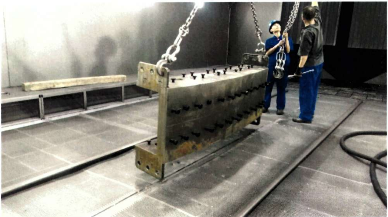
Figure 8b. – Span support segment after blasting
