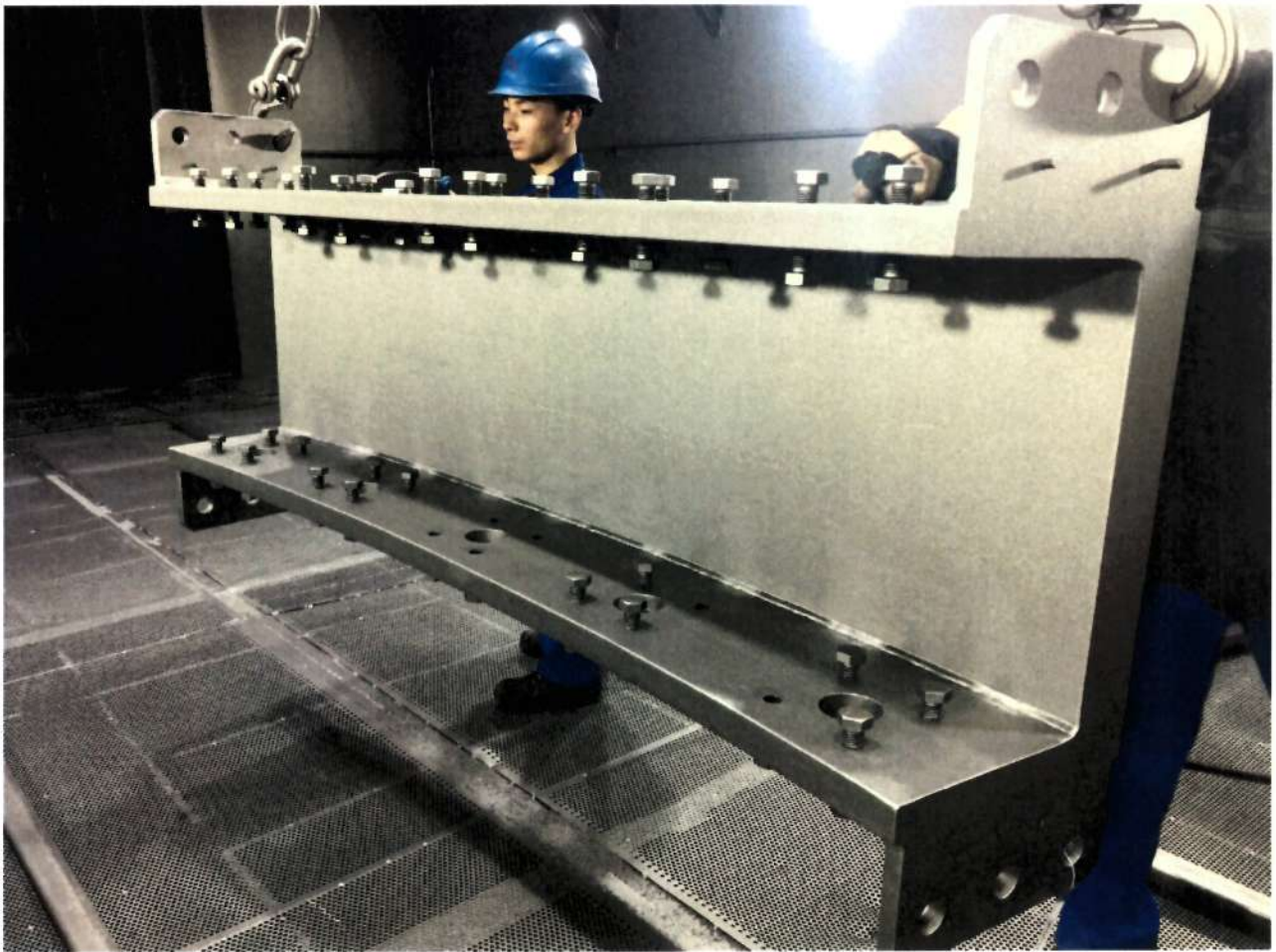
Figure 8c. – Span support segment after blasting
