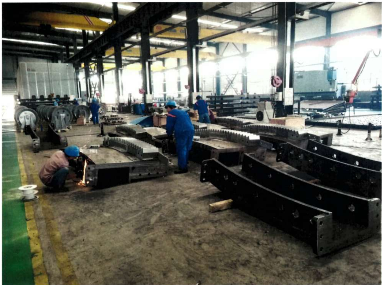
Figure 7a. – Span support segments
