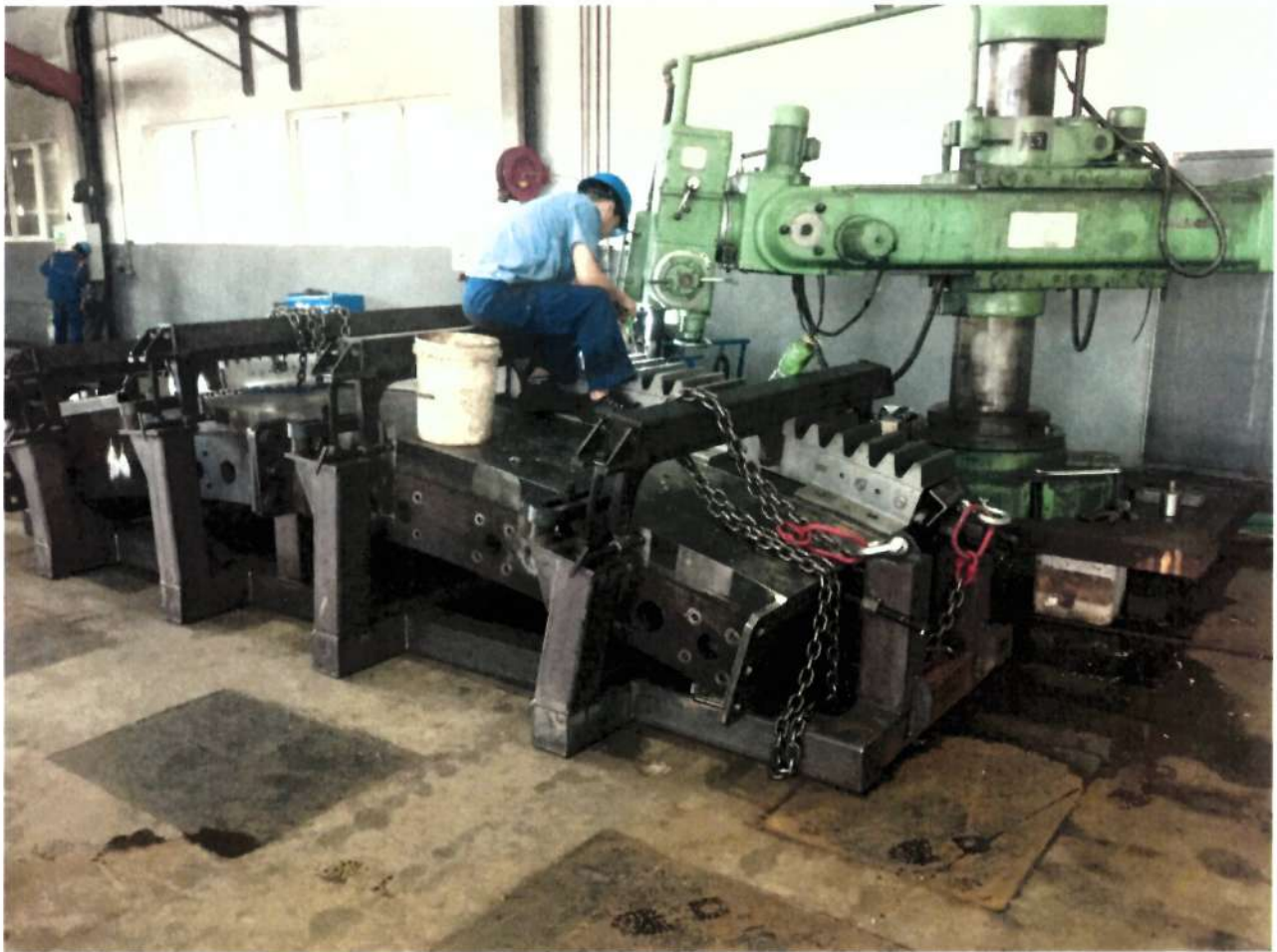
Figure 6a. – Angle hole drilling – north truss
