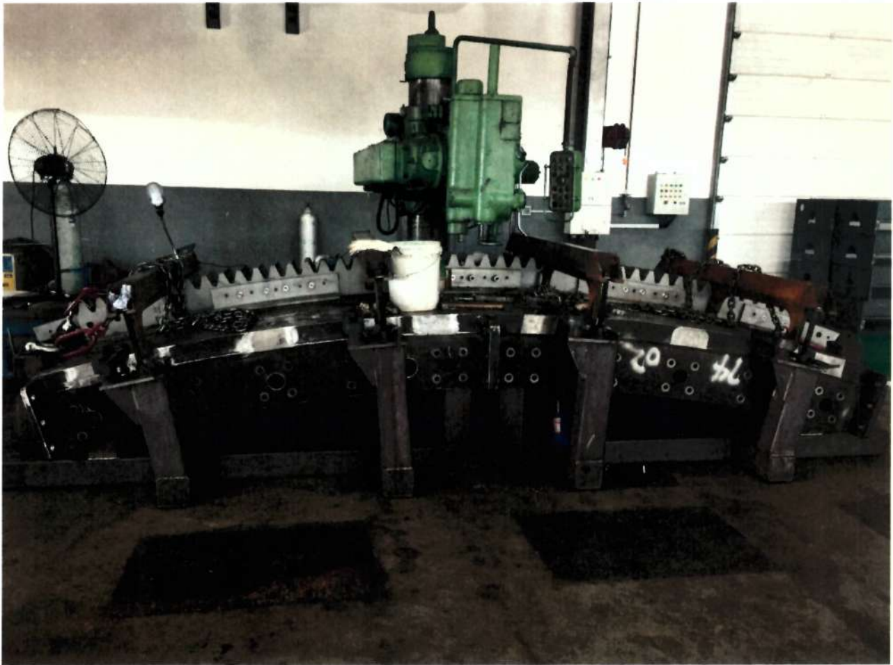
Figure 6b. – Angle hole drilling – north truss
