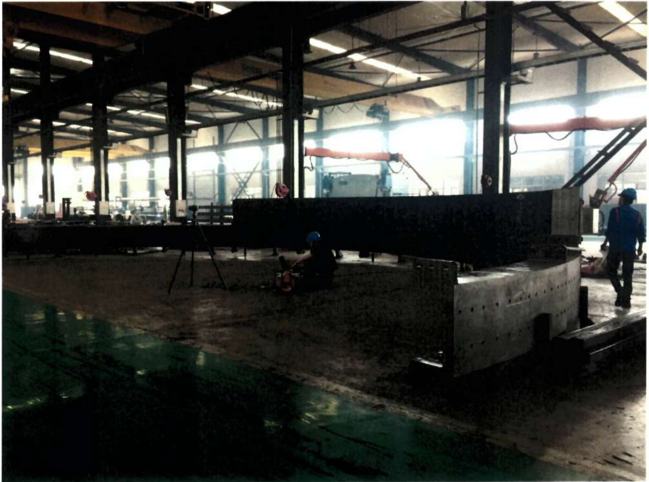
Figure 7c. – Trial fit up of span support structure
