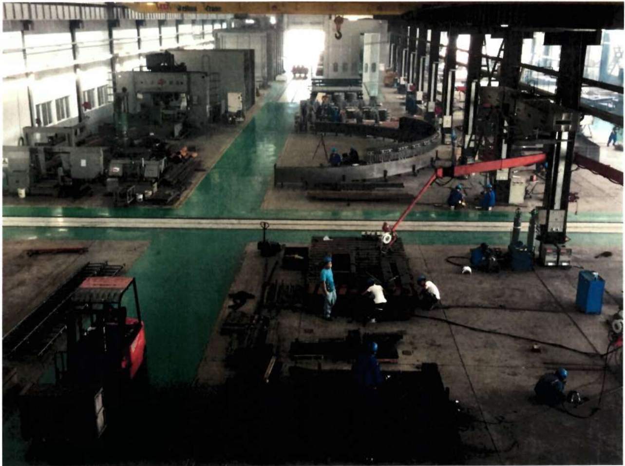
Figure 7d. – Fit up of Span Support Structure
