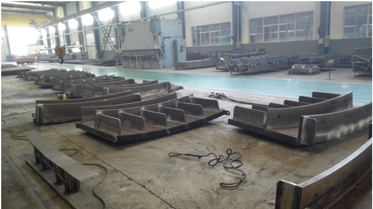
Figure 6 - Completed Span Support Segments
