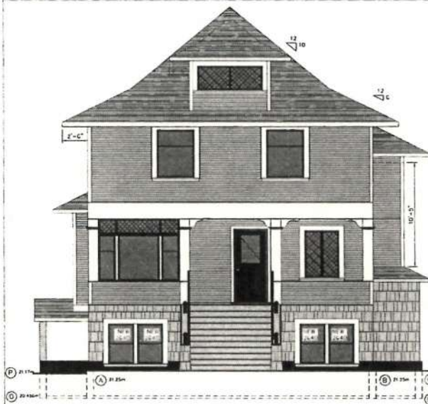
PROPOSED EAST ELEVATION
