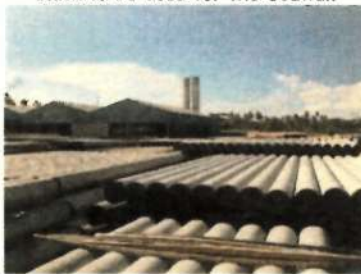
5: Concrete Pilings painted black to be used for the Seawall
