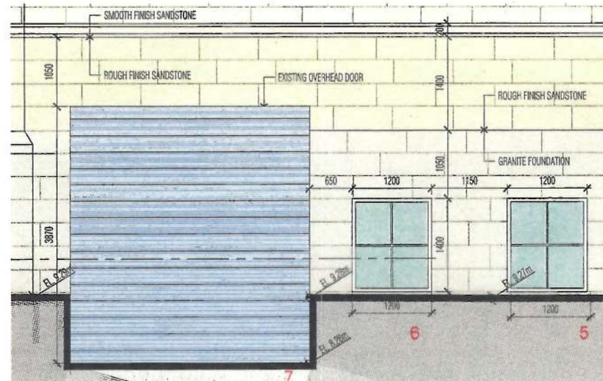
EXISTING SOUTH ELEVATION - GROUND FLOOR OPENINGS 5, 6 & 7 SCALE 1:50
