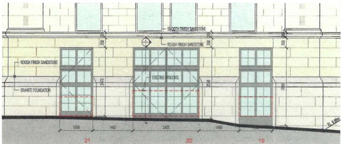
PROPOSED NORTH ELEVATION - OPENINGS 19, 20 & 21 SCALE 1:50
