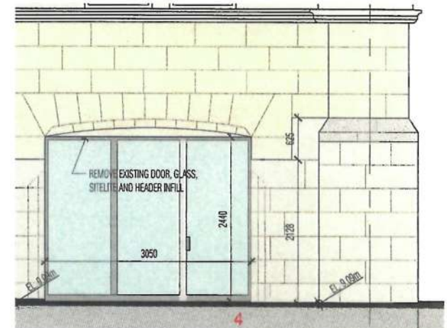
EXISTING WEST ELEVATION - GROUND FLOOR OPENING 4 SCALE 1:50
