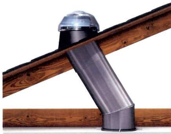
Figure 1: A roof cross-section showing the traditional application of a “solatube” to bring light into a building.
