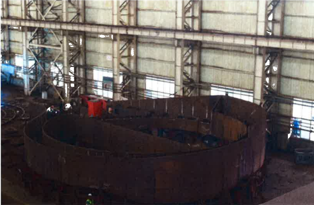
Photo 4 – Lower counterweight welding in progress
