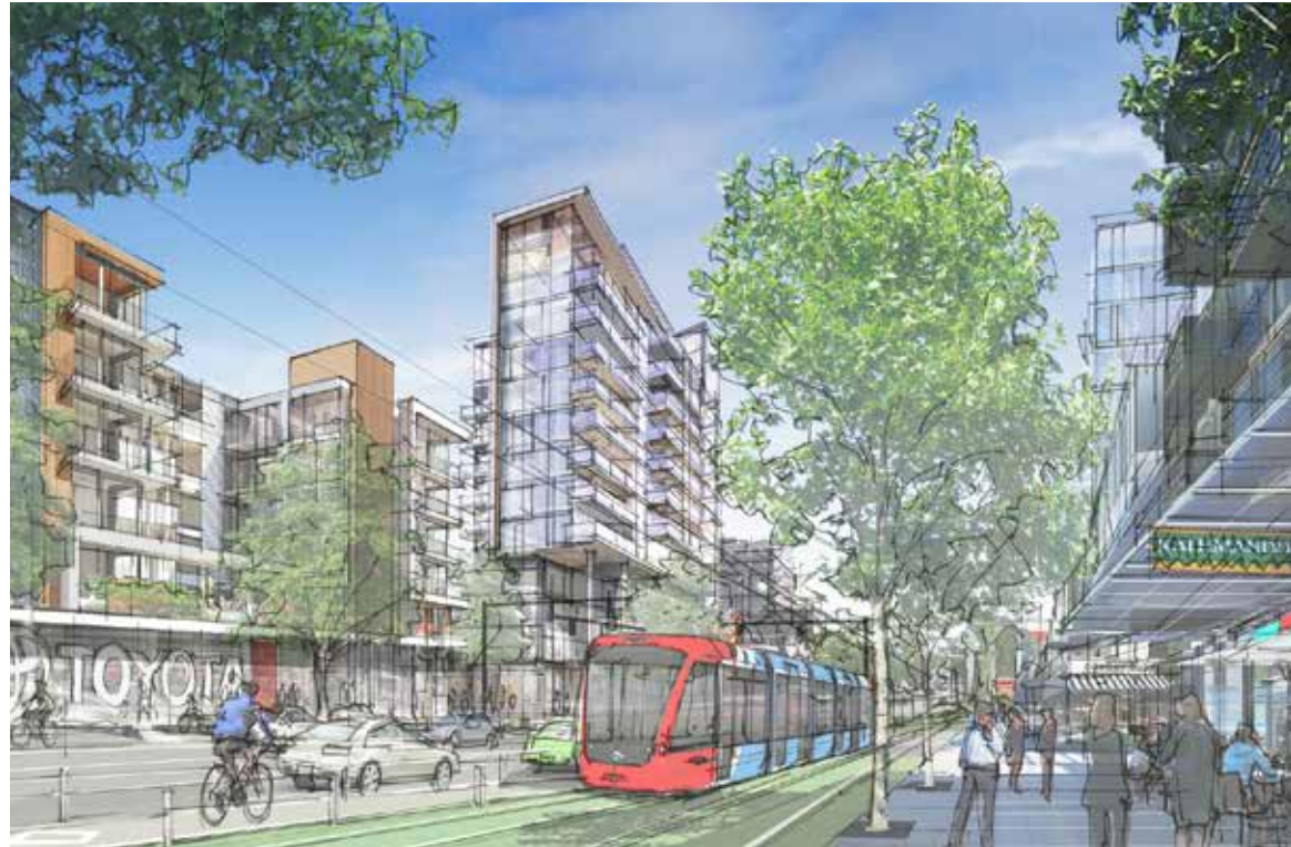
Figure 9: Concept drawing showing an example of a frequent transit route through a Town Centre, with enhanced sidewalk and protect bicycle lanes framed in by tall buildings. In this example, Light Rail Transit (LRT) is shown with tracks along the side of the right-of-way, although centre lane is another common case for LRT.
