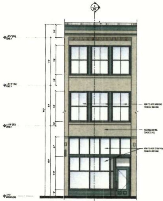
1 ELEVATION: RESTORED FACADE BAY scale: 1/4" = 1'-0"
