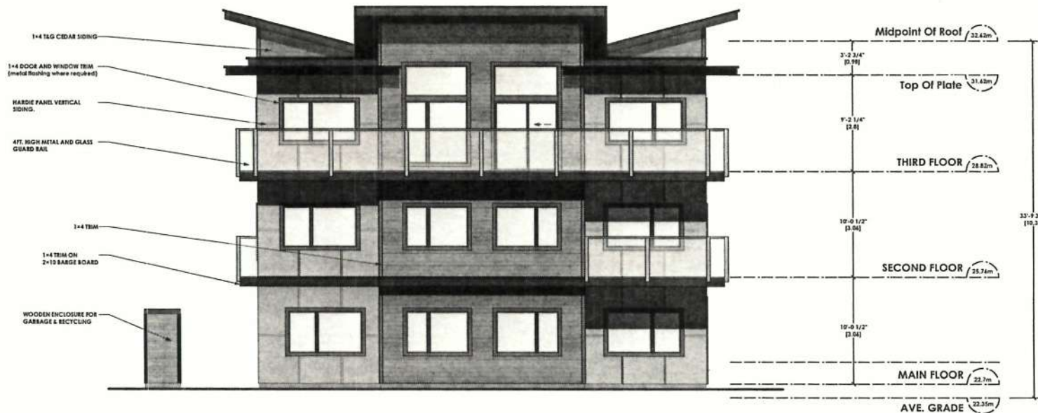
1 EAST ELEVATION (RICHMOND RD. SIDE) A6 Scale: 1/8" = 1'-0"
