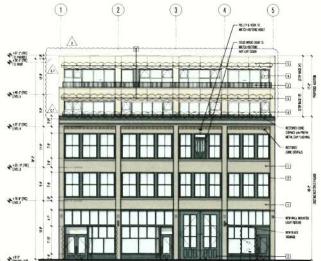
3 PROPOSED FRONT ELEVATION (RESTORED TO HERITAGE) SCALE: 1/8" = 1'-0"
