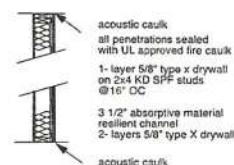
WALL TYPE E UPGRADED RATED EXISTING PARTITIONS ASSEMBLY W4A 1 HR RATING, STC 51
