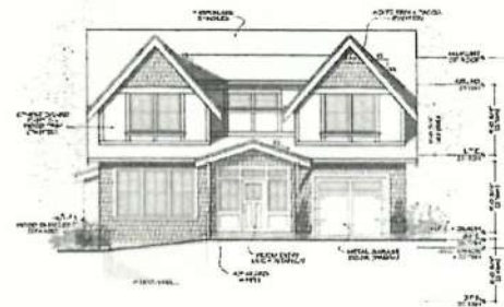
○ Lot B - Front (Oakland Ave) Elevation Scale: 1/8" = 1'-0"
