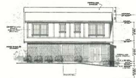
○ Lot B - Rear Elevation Scale: 1/8" = 1'-0"
