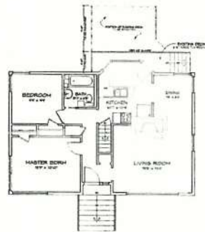
Lot A - Main Floor Plan Scale: 1/8" = 1'-0"
