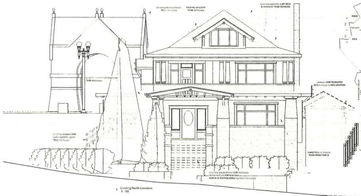
EXISTING ELEVATION SHOWING GRANITE STONE FOUNDATIONS & PILLARS
