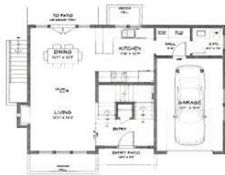
○ Lot B - Main Floor Plan Scale: 1/8" = 1'-0"
