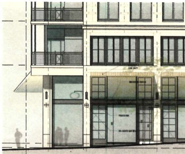
SOUTH DETAIL ELEVATION - GOVERNMENT STREET SCALE 1:50
