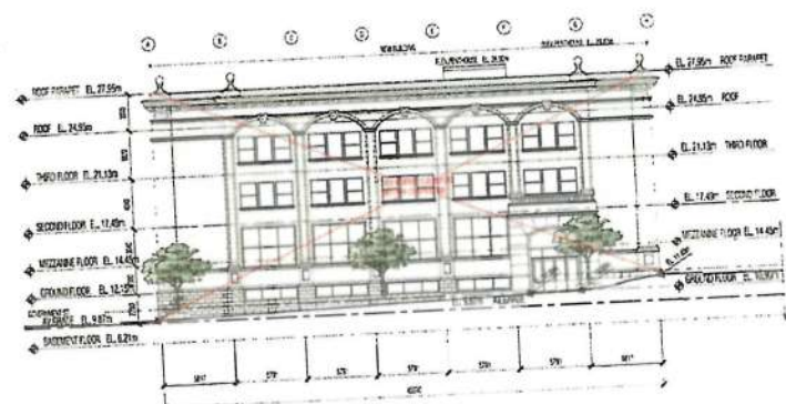
EAST ELEVATION CONTEMPLATED ALTERATIONS TO WINDOW OPENINGS SCALE: 1:200
